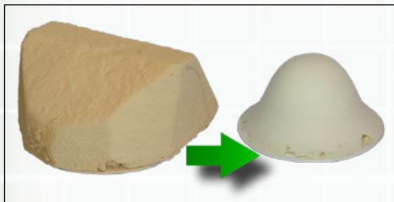
1. I constructed the domed roof from an offcut of insulating foam glued to a card disc. The foam was far from the correct shape and needed some work. First, I trimmed it with a large knife, then sanded it down with abrasive paper and sanding sticks until I had the unique domed shape. The sanding was a little messy, so this was done in the garden rather than in the workshop.
