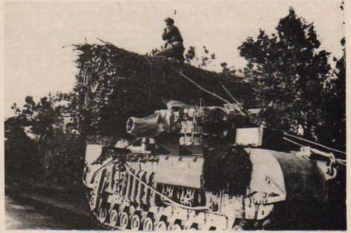
A Churchill AVRE with the fascine mounted on its front reduced visibility, hence the commander riding on top of it. Note spare track links on the turret for extra protection. (RAC Tank Museum)
